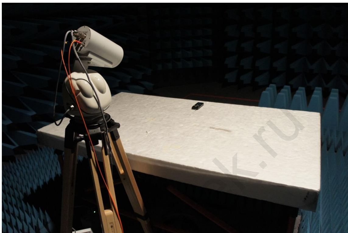
Picture 5: Test setup radiated immunity test
