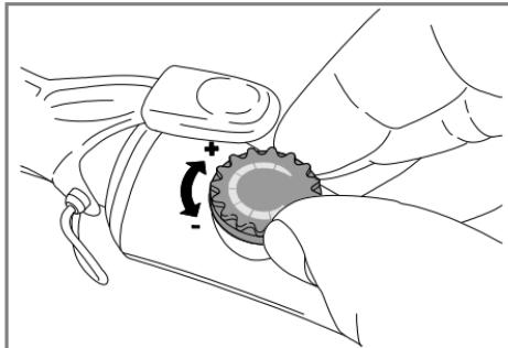
The temperature can be adjusted continuously.
