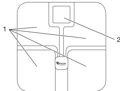
\*ITO (indium tin oxide): this innovative conductive coating acts as an electrode for the body measurement.
